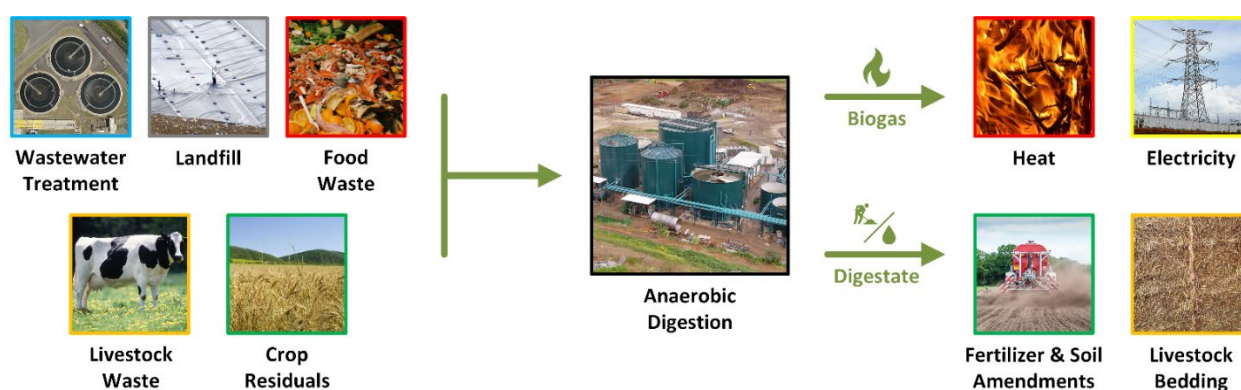
Figure 5: Biogas production can use many types of waste streams to produce heat and electricity.
