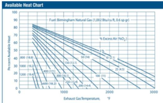
Determine the available heat under present and desired conditions by reading up from the flue gas temperature to the curve representing the excess air or O<sub>2</sub> level; then, read left to the percentage available heat (AH)
