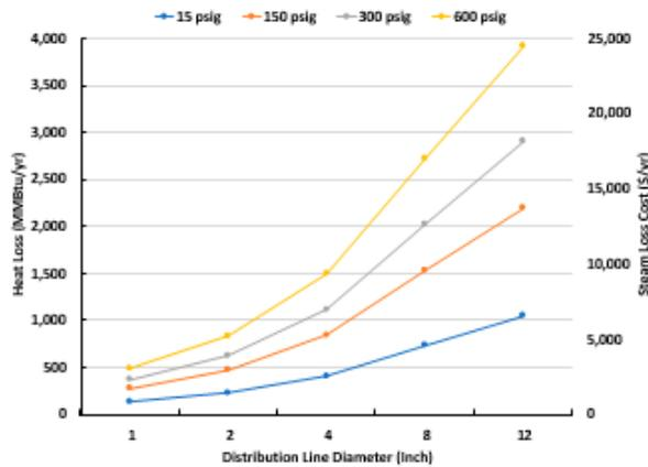
*\*\*Based on Natural Gas unit rate of \$0.5/therm and boiler efficiency of 80% and 8,760 operating hours per year.*
