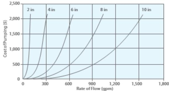
\*Based on 1,000 ft. for clean iron and steel pipes (schedule 40) for pumping 70°F water. Electricity rate of 0.05 \$/kWh and 8,760 operating hours annually. Combined pump and motor efficiency of 70%.
