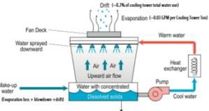
Blowdown (~0.006 GPM per Cooling Tower Ton @ 6 Cycles of Concentration)
