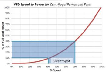
\* Avoid running VFDs fully loaded by setting maximum speed to ≤90%.
