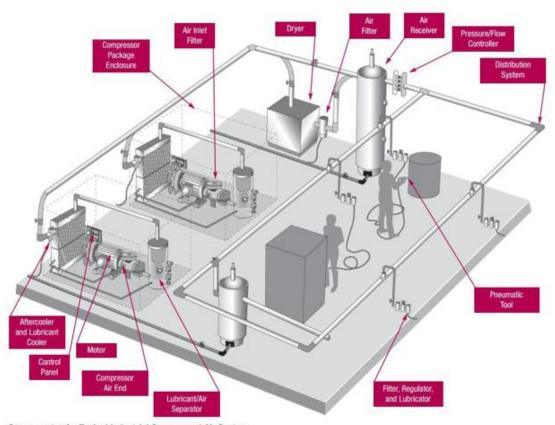
Components of a Typical Industrial Compressed Air System.
